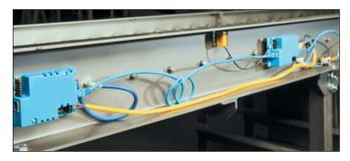
All electrical controls are self-contained within the side frames, which eliminates the need for wiring back to PLCs, thus reducing the cost of field wiring as well as wear, contact damage and maintenance. The PosiGrip is ideal for both clean environments and tough, rugged applications.
