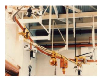
These systems are offered in capacities ranging from 50 pounds (or less) to 6,000 pounds per carrier with carrier production rates up to 80 carriers per hour. Ask for our detailed component catalogue or a system engineer to evaluate your needs.
